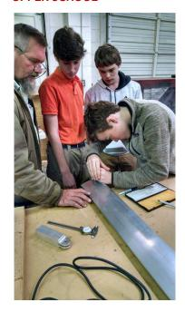
The Fuqua School aviation class is currently securing the wings on the fuselage before moving to the final step of outfitting the cockpit. Students are focusing on precision drilling along the wing struts which requires skills in new tools and advanced mathematics. The wings and their supports are arguably the most important part of the plane so the process of attaching them has been carefully guided by the volunteer build experts.
