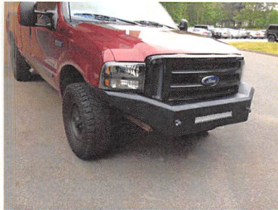
Senior Project: CAD designed truck bumper cut on plasma cutter
