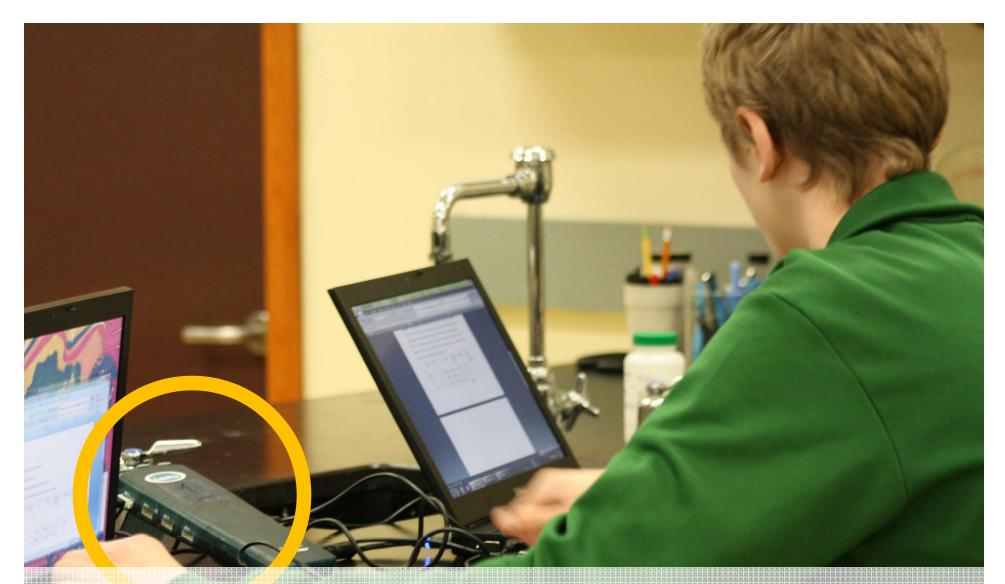
Peter Clark's students measure sound pressure by using microphones connected to laptops and Vernier LabPro data collectors.
