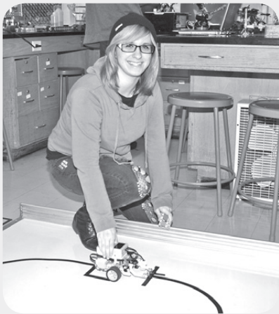
Madison Berryann, a senior, tests a robot she created for an assignment called the Container Challenge. The robot is programmed to pick up a "crate" and then use its sensors to carry the crate to a specific location like a common warehouse robot.
