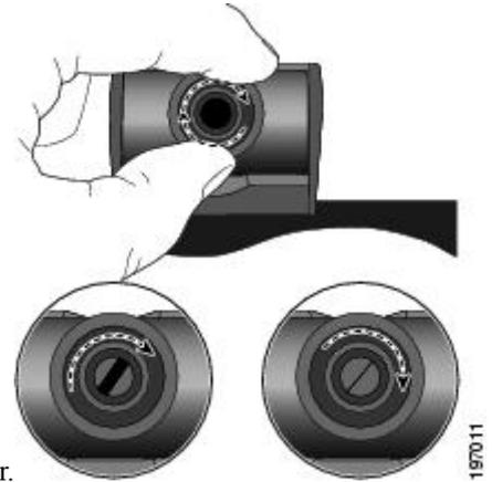
The following figure shows the location of the camera lens shutter.
