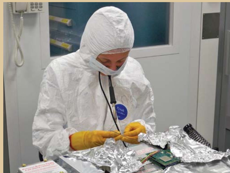
In the NASA clean room, Nina solders one of her experiments to the base plate that will be attached to the space station.
