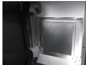
6-8 Hold the UV lamp, pull it up and remove it from the UV lamp holder.
